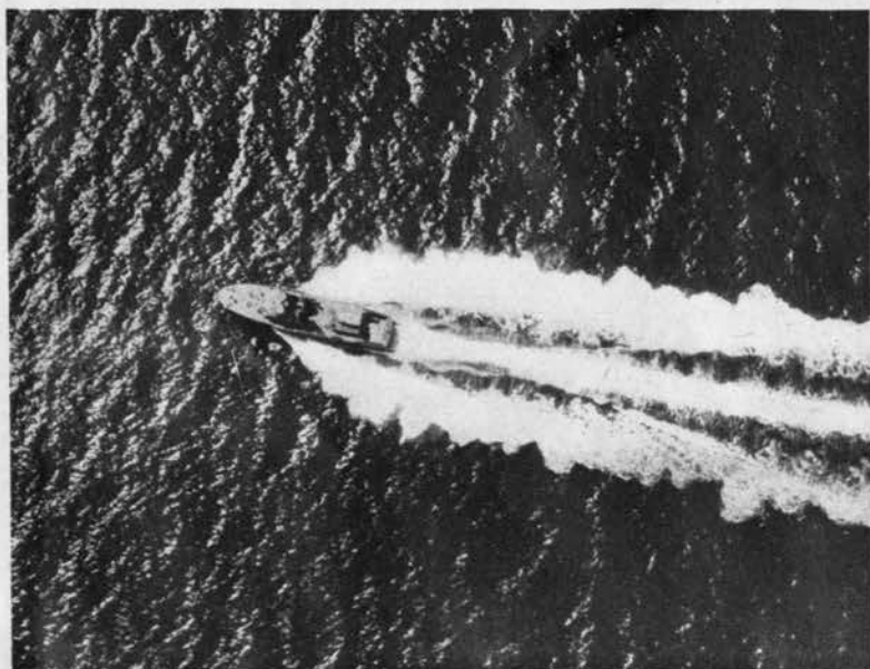
Elliptical hull , machine-gun position atop cabin and a large deck break at the stern mark the 63-ft. rescue boat. Sometimes employed as patrol vessels, the 63-footers may be seen as far as 250 miles out from land.
